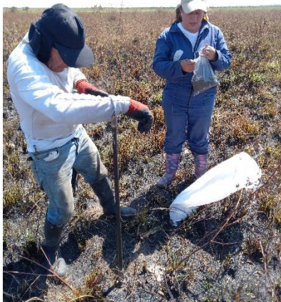
Photograph 3-2. Use of drilling for soil samples and analysis of organic carbon and fine roots
