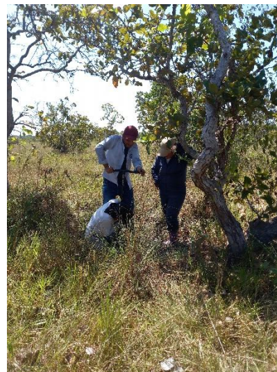
Photograph 3-2. Use of drilling for soil samples and analysis of organic carbon and fine roots
